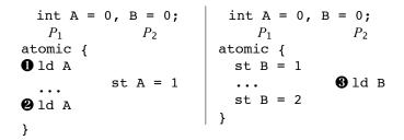
Fig. 2. A strongly atomic semantic must provide both *non-interference* and *containment* with respect to non-transactional code. Non-interference (left) prevents **0** and **2** from observing different values. Containment (right) prevents **3** from observing the internal value 1.
