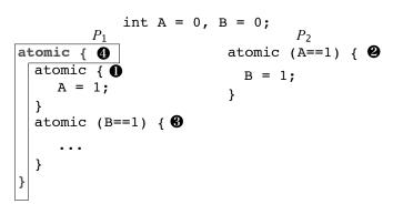
Fig. 4. A program that executes correctly when the boxed atomic block is not present but deadlocks when the atomic block is introduced to compose the two transactions it contains (**0** and **3**).
